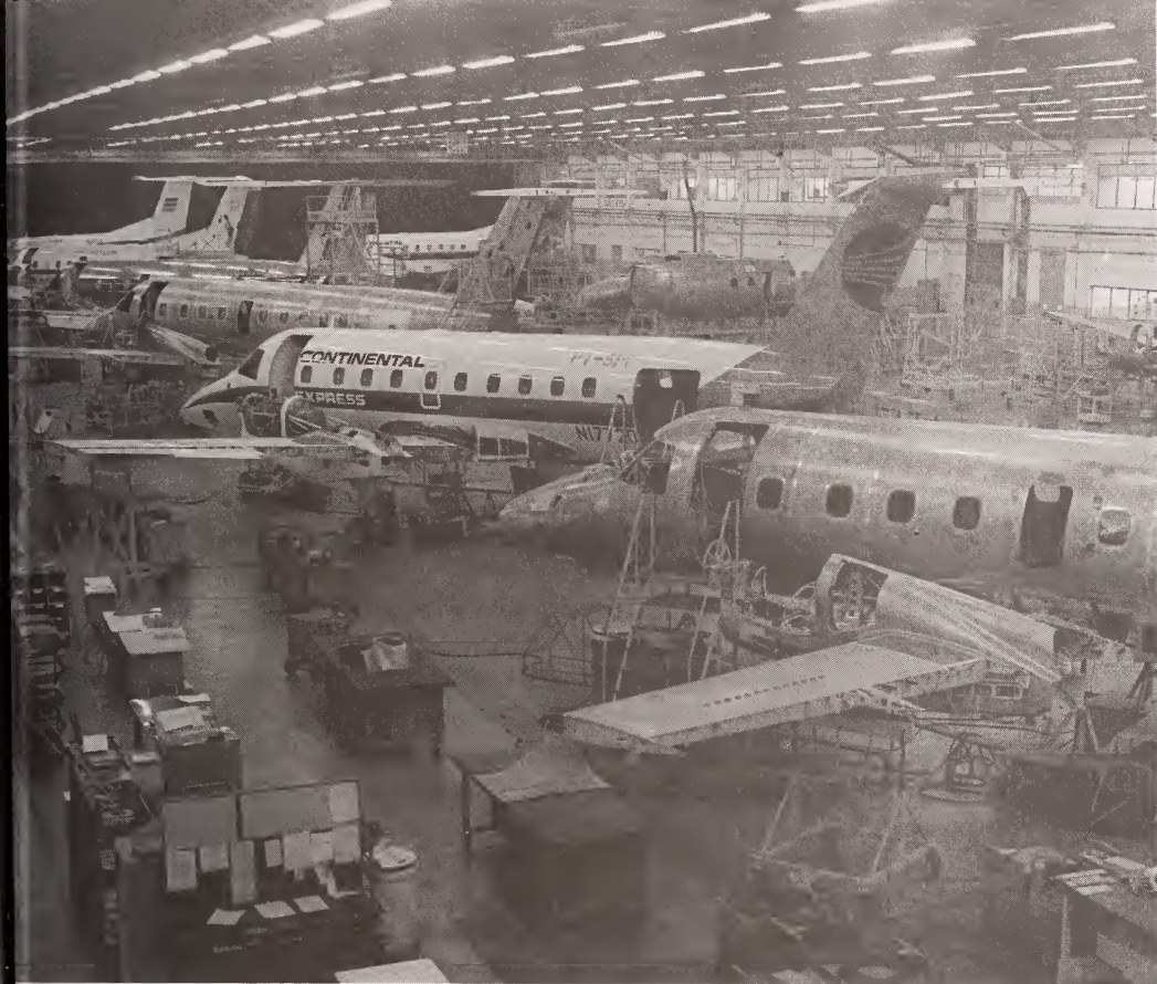
An Emb-120 Brasília on the final assembly line at the factory of the Brazilian Aeronautics Company (Empresa Brasileira Aeronáutica—Embraer) in São José dos Campos, São Paulo State Courtesy Embraer
